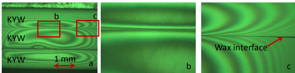
Fig. 2.19. Visualization of rounding of the polished end-facet of a stack of three KYW samples. The fringes are formed between a glass cover slide that has been placed on top of the polished interface, hence these images are taken through this glass substrate, illuminated with green light.
